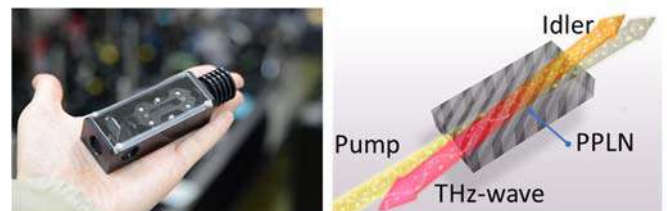
Fig. 1. (Left side) Photo of the backward THz-wave parametric oscillator. (Right side) Schematic illustration of the backward THz-wave parametric oscillation using a slanted stripe-type PPLN. The yellow, orange, and red arrows show propagating direction of the pump, idler, and THz-wave, respectively.
