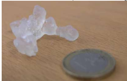
Figure 1: Upscale aggregate realized in acrylate resin ( \epsilon_r = 3 + j*0.1 ) with an additive fabrication printer based on Stereo Lithography (SL)
