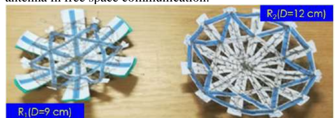
Figure 1: Photograph of the parabolic textile reflectors: R_1 ( D=9 cm, in left) and R_2 ( D=12 cm, in right).
