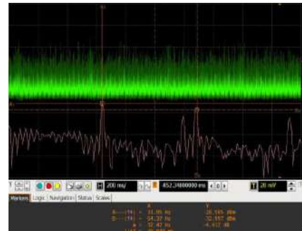
Figure 11. Oscillogram for the Ethernet interface during data transmission (transmission of a 100MB file) with transmission intervals of 30 ms. The signal received by the antenna for f = 1,453 GHz given from the VIDEO output of the FSET22 receiver
