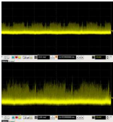
Figure 9. Oscillogram for the Ethernet interface during data transmission is on. The signal received by the antenna for f = 1.73 GHz given from the VIDEO output FSET22 receiver
