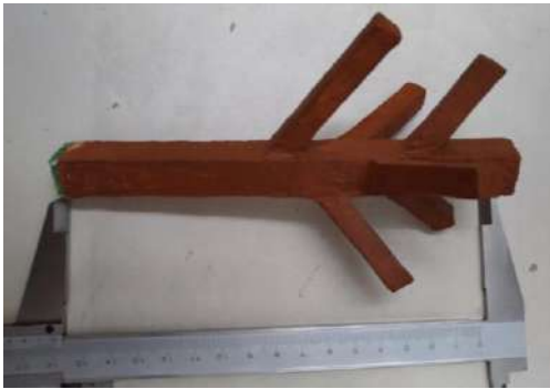
Figure 2: Downscaled tree realized in PLA with a Fused Deposition Modeling (FDM) 3D printer and filled with a liquid (glycerol plus water) having a permittivity of \epsilon'_r=8 to 10 and \epsilon''_r=6 to 9 in the considered frequency range.
