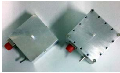
Fig. 2 Photograph of the transient E-field sensor
