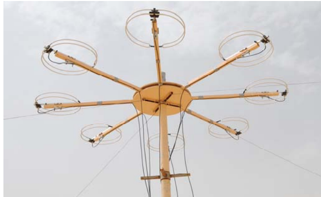
Figure 1: An eight element circular antenna array for VHF radio signals.
